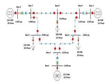
Fig.2 9 bus system 3 generators with increase load
