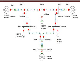
Fig.3 9 bus system 3 generators with further increase load
