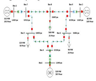
Fig.4 9 bus system 3 generators with further increase load
