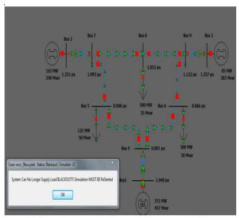
**Fig.5** sudden increse load on Bus no 6, Removal of line Load is suddenly increase on bus number 6 from 90MW to 300MW now system goes in total blackout this is clearly shown in figure 5. When load is increased on bus number 6 above from 100MW at that time we have to start to trip the line connected to bus number 5, and finally we remove bus number 6 also to maintain stable power system this we forecasting power blackout that is shown in figure 5.
