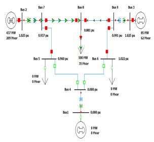
Fig.5 Normal system opreation on redused load
