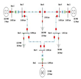
Fig.1 9 bus system 3 generators in Initial condition
